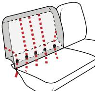
If the backrest is attached to the vehicle frame, your covers should be open backed. To make room for the straps to drop between backrest and vehicle frame, pull the cushion up. Often, this will force the backrest to move forward from the frame.
