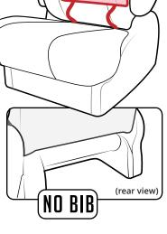
If your hand can pass through to the back between the backrest and cushion, your seat has no bib. Your backrest cover will have a carpeted tab and a velcro strip on the back. Push the front tab between the backrest and cushion to the back, and attach to velcro.
