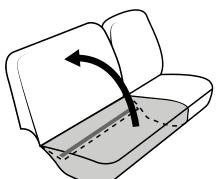
During cushion cover installation, flip seat(s) up while tucking the velcro flap
