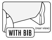
If your hand can't pass through to the back between the backrest and cushion, your seat has a bib. The backrest cover will have straps on the front tab and elastics/velcroon the back. Push the straps between the backrest and cushion, and below the cushion towards the front, and then attach them to the inner buckles. Attach the velcro strip at the back to the carpeting on the seat. Or, if there are elastics, attach them using the "s" clips to the underside of your cushion.
