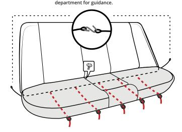
Insert straps into their corresponding buckles. Pull the chord by their loops together, and connect with an "s" hook. Pull straps downwards to tighten.
